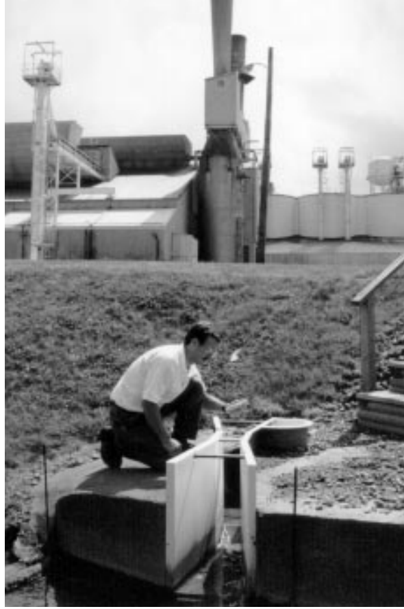
PPG Industries Inc. works: Meadville, PA. Plant Environmental Engineer checking the pH of discharge water from plant operations.
